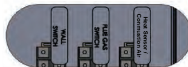
Control box LED lights
