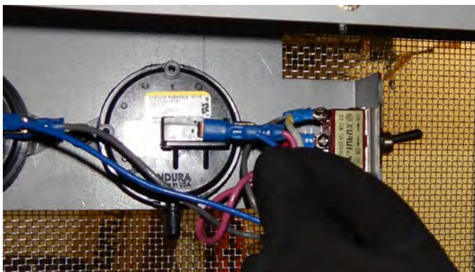
Figure 112. Disconnect blue wire.
