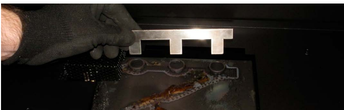
Figure 23.d Pushing the Rock Guard down into place.
