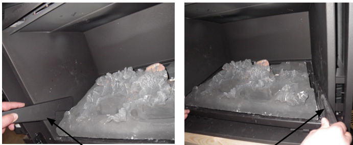
Diagram 2 Left /right filler sections
