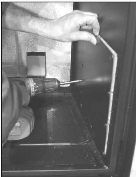
Figure 13: Removing Access Cover.
