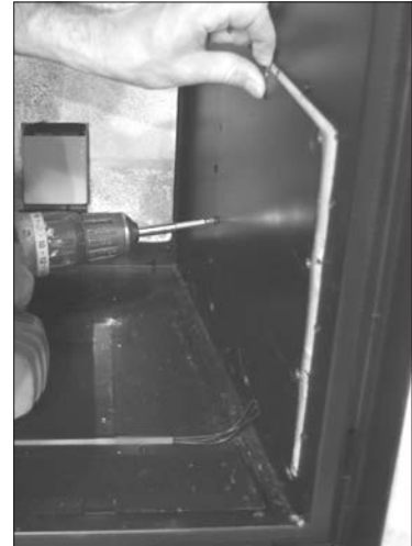
Figure 57: Removing Access Cover.
