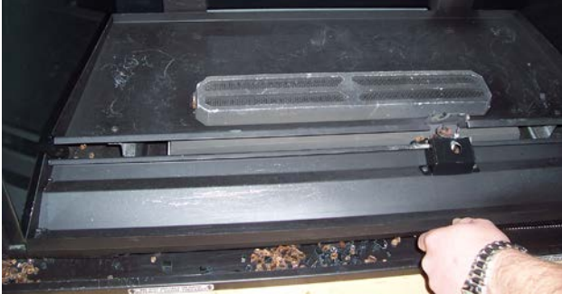
Figure 63: Lift Out Front Panel
