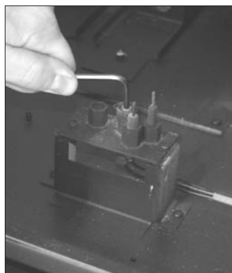
Figure 53: Removing the Pilot Orifice.
