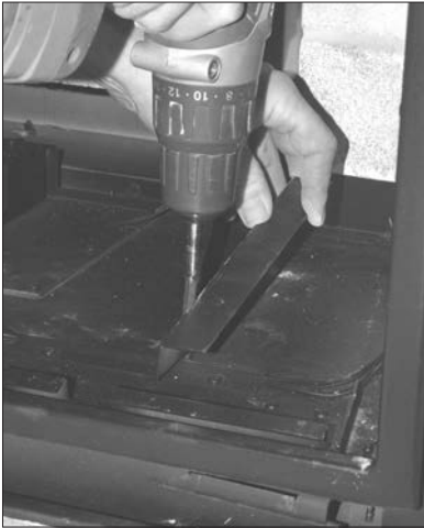
Figure 56: Removing the Right Burner Support.
