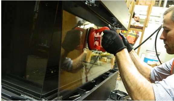
Handle front panel with supplied vacuum clamps
