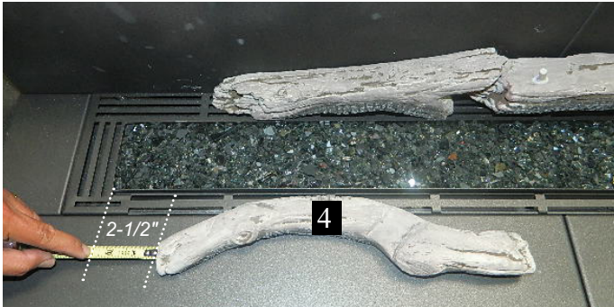
Log 4 to edge of burner
