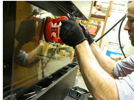
Handle front panel with supplied vacuum clamps
